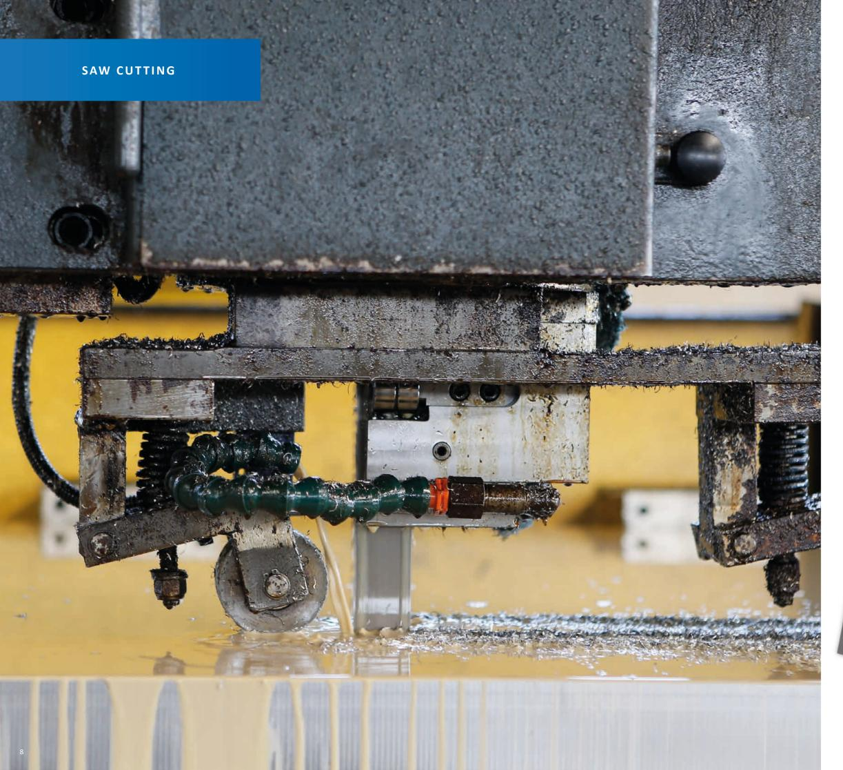
Saw cutting is the solution for machining medium and large thicknesses from 8 mm and higher.
